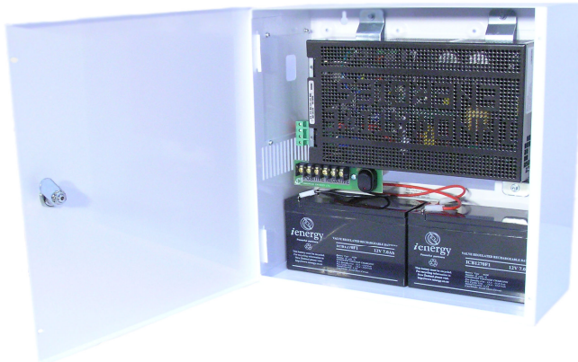
SN27/10SA shown, includes distribution terminals
