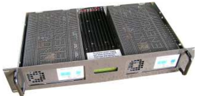
2U rack with 2 x SR250D12 power supplies and decoupling diodes on heatsink plus V/I meter
